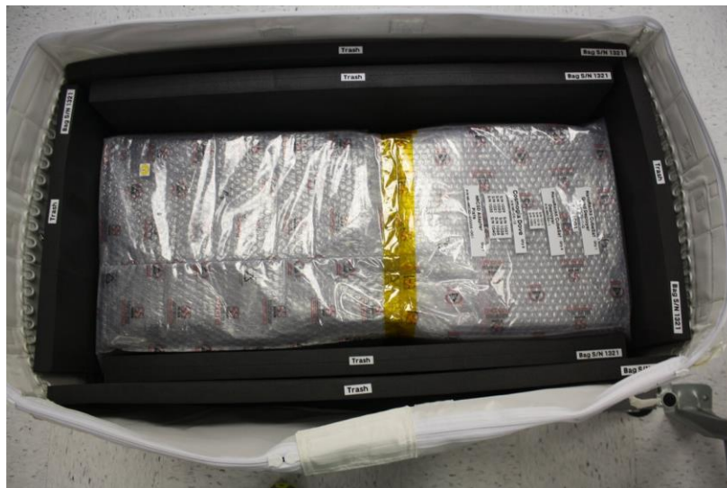
Figure 3.4.2.7-1: Sample NRCSD Stowage Configuration for Launch (NRCSD Quad-Pack in M2 CTB)
